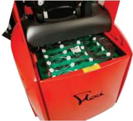
Low lift off or roll off for fast changes if needed. No service components or motors underneath.
