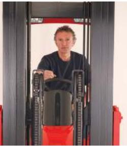
FLEXI operators have excellent visibility thanks to a standard 'Hi Vis' lift mast which has four side mounted lift cylinders. Mast tilt allows easy fork entry into pallets - even on lorries.
