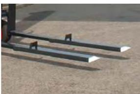
Telescopic double deep fork version provides extra 50% storage capacity over reach trucks for true bulk store operations.
