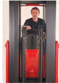
Operators have excellent forward visibility thanks to the triplex free lift mast, with its twin side mounted lift cylinders. Safe forward pallet pick up and set down.
