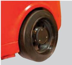
Cushion tyres allow operation on standard warehouse floors. Low point loadings compared to guided VNA trucks.
