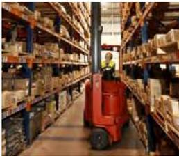
Chassis in 1250mm and 1350mm wide options allow higher lifts with heavier loads. AC power for fast travel speed.
