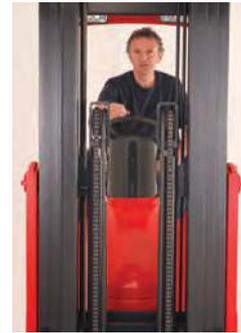
Operators have excellent forward visibility thanks to the triplex free lift mast, with its twin side mounted lift cylinders. Mast tilt means easy fork entry into pallets - even on road trailers.
