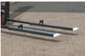
Telescopic double deep fork version provides up to 50% extra storage capacity over reach trucks.
